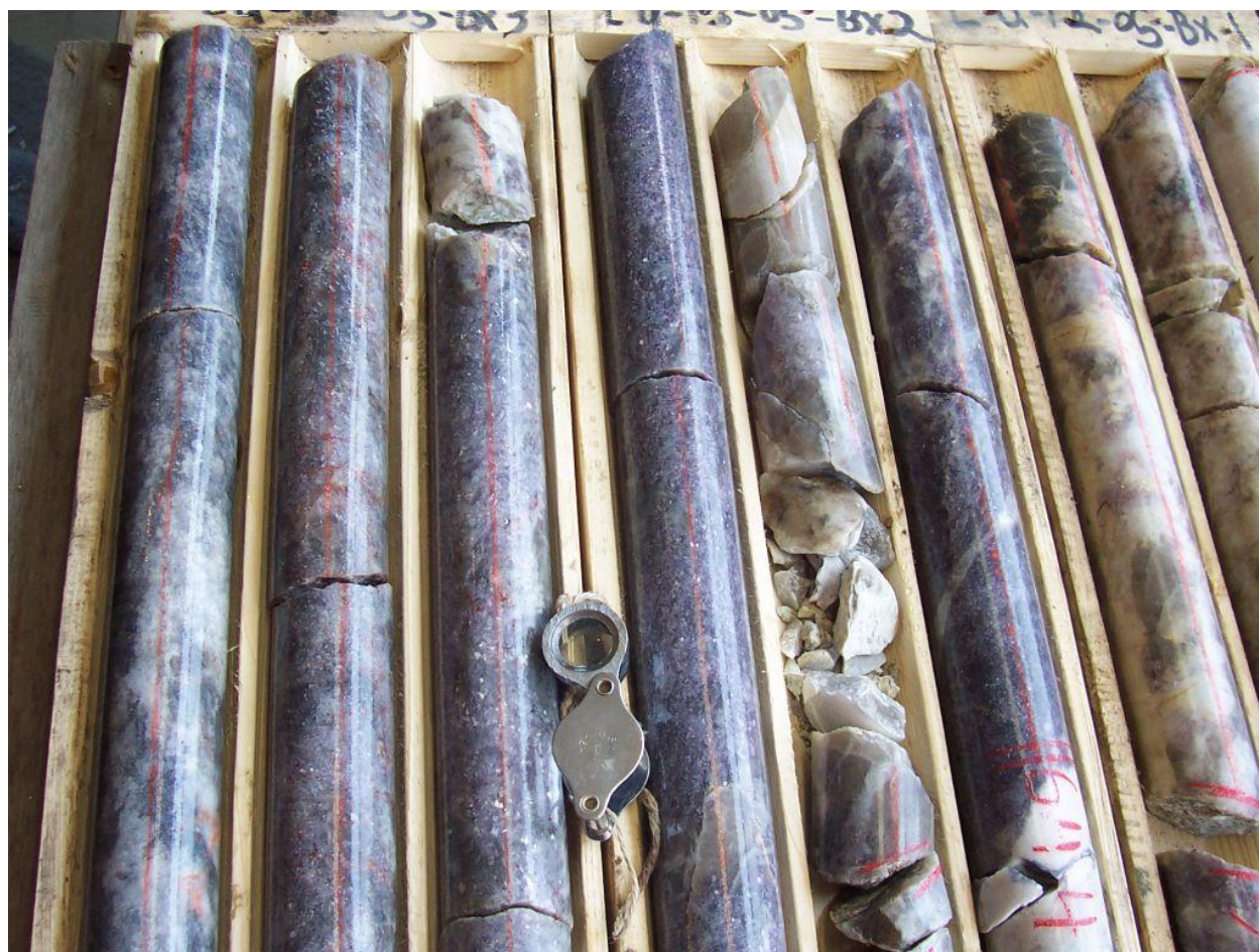
Photo 3. Lepidolite-albite lithology in upper fractionated zone from drill hole LU-12-5 on Lucy North Dike (March, 2012).
