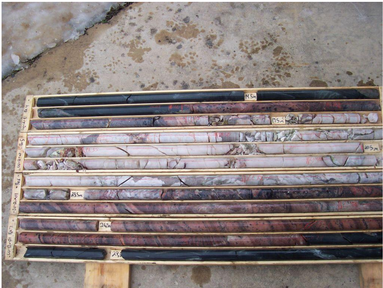
Photo 2. Core intersection of Lucy South Dike from hole LU-12-1 showing white coloured upper fractionated zones and lower pink coloured poorly-fractionated banded aplites and wall zones (March, 2012).
